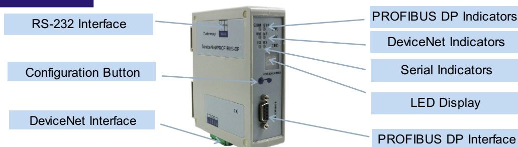
PROFIBUS DP network status lights (COM, SYS)
