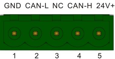
Note: Voltage between 24V+ and GND is 24V, power range is 11~30V;
