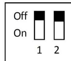
The DIP switch is located at the bottom of the gateway, bit 1 is debugging bit and bit 2 is configuration bit.
